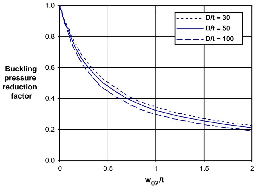
**Figure 6** Reduction factors on two-lobe buckling pressure due to symmetrical gap imperfection expressed as a function of gap/thickness ratio
