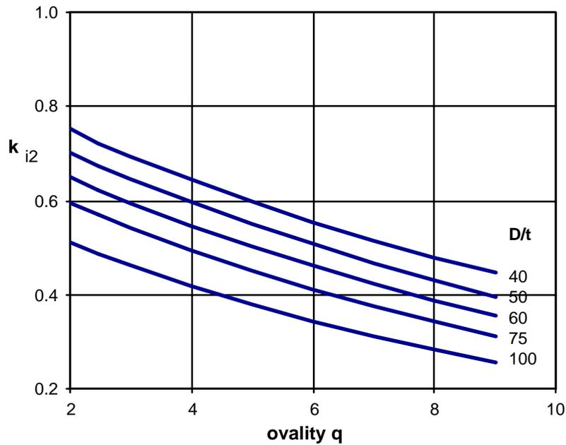
**Figure 9** Combined imperfection factor on 2-lobe buckling pressure of perfect circular liner as a function of system ovality, for characteristic gap imperfection of 0.5%
