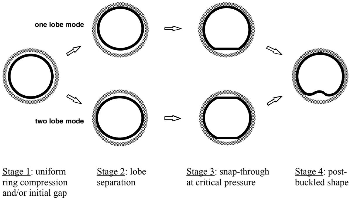
**Figure 4** Steps in non-linear hydrostatic buckling of encased circular liner pipe (liner deformations fully consistent with boundary conditions)
