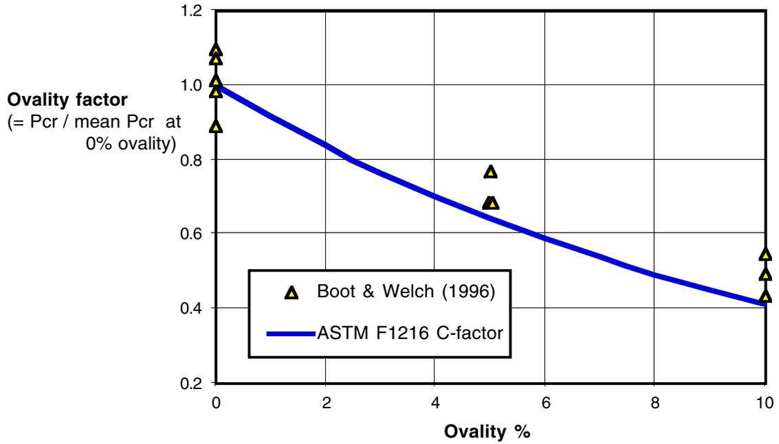
**Figure 3** Experimental ovality factors for liner of  $D/t = 45$  compared with ASTM C-factor
