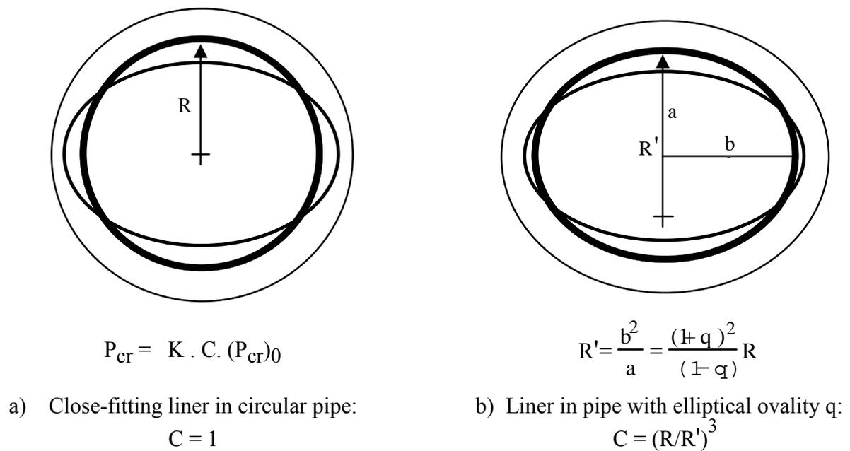
**Figure 2** Liner deformations implicit in current ASTM design formula based on linear theory of unrestrained buckling with enhancement factor K and ovality factor C
