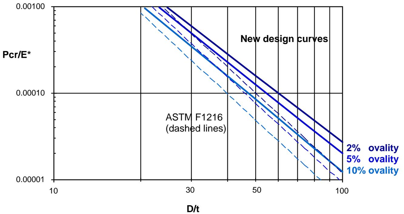
**Figure 8** Typical form of new design chart for CIPP incorporating a characteristic gap imperfection (here 0.5%)
