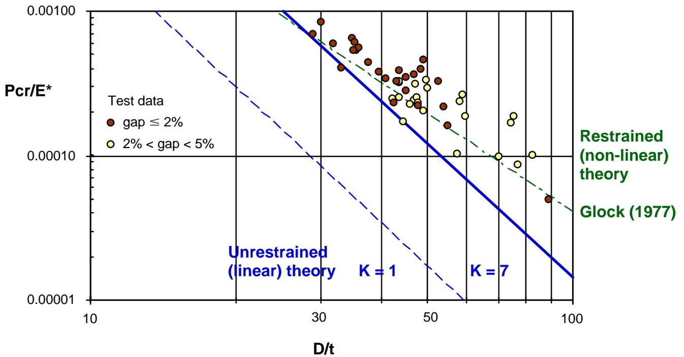
**Figure 1** Aggarwal's 1984 hydrostatic buckling data compared with contemporary theories
