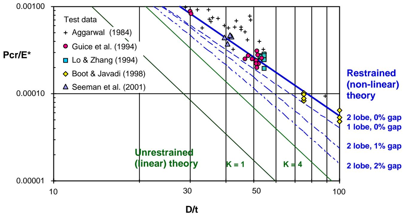
**Figure 5** Various gap-corrected hydrostatic buckling data compared with current theories for perfectly close-fitting, perfectly circular liners
